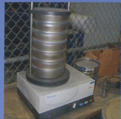
J878.09- 8" Laboratory type sieve shaker by RETSCH as model AS200.
