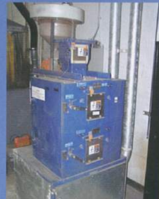
J878.05- Roll Mill by MODERN PROCESS EQUIPMENT. Two (2) levels each with two (2) rolls per level .
