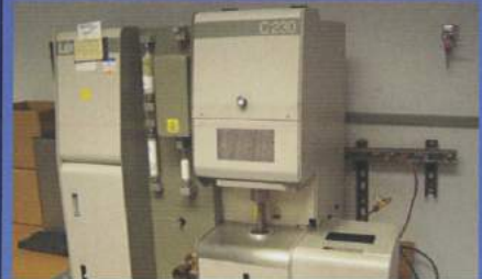
J878.44 - CARBON DETERMINATOR - LECO 230
