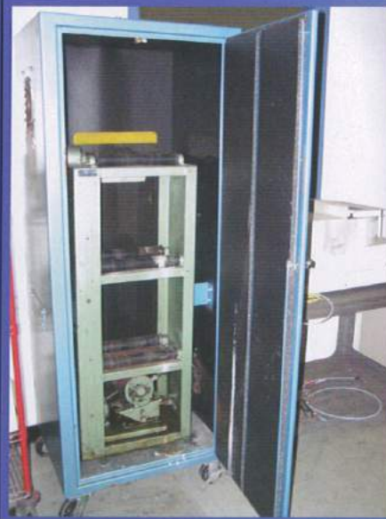
J878.35- JAR MILL with three (3) tiers each tier with two rollers twelve inch (12") long.
