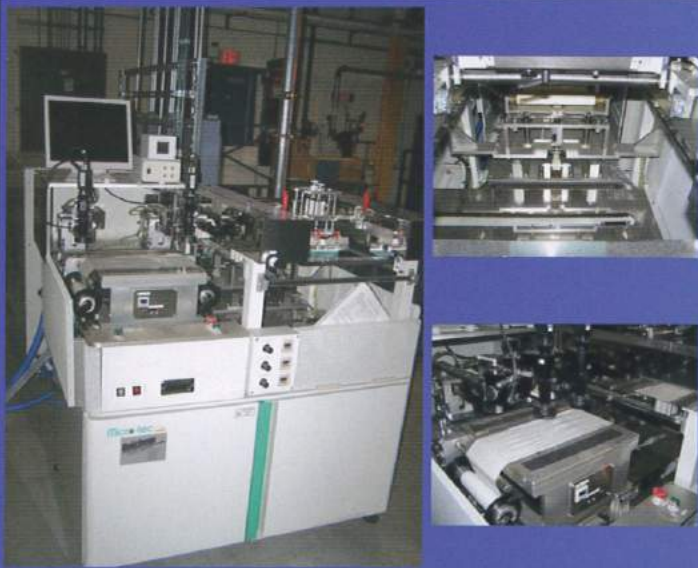
J878.57- Low-pressure screen printing machine by Micro-Tec Co. Ltd with maximum printing area 230 mm x 250 mm (approx).
