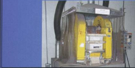
J878.06 - JAW CRUSHER by Pyro Systems 3000-040. The jaw opening is 6" x 6".
