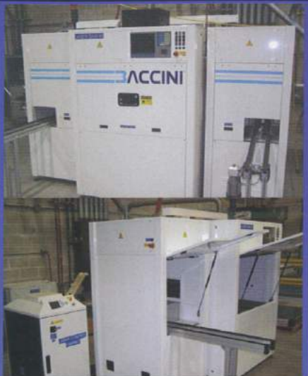
J878.53 - LASER SAW by BACCINI For advanced wafer etching and processing. New in 2006.
